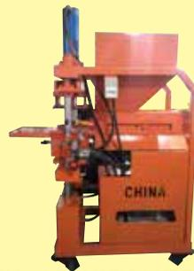
SEMI-AUTOMATIC HYDRAULIC CLAY BRICK MAKING MACHINE (Sy2- 10)
