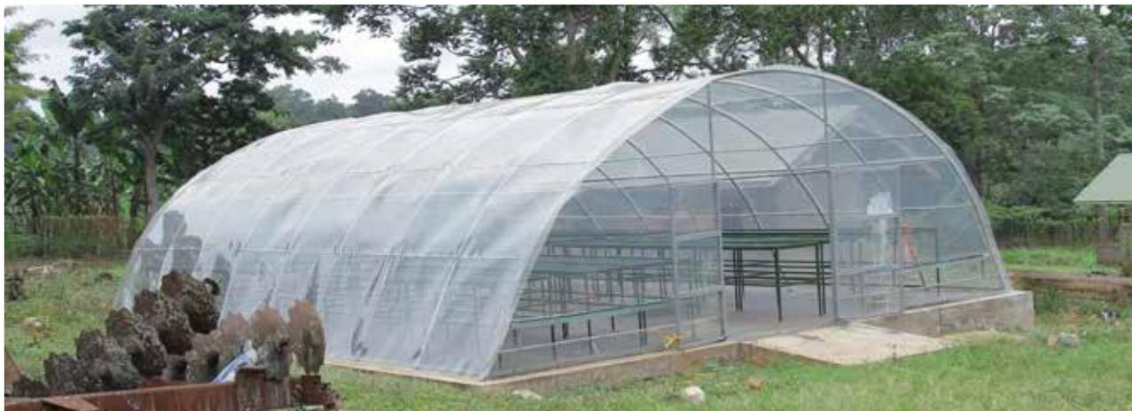
**Figure 70(a).** Large scale solar drier
